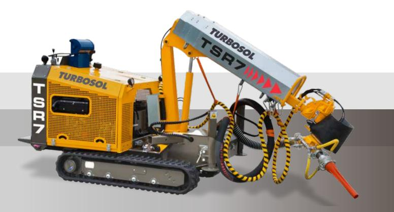
TSR 7: crawler equipment designed for shotcrete applications in jobsites with difficult access and tunnels.
